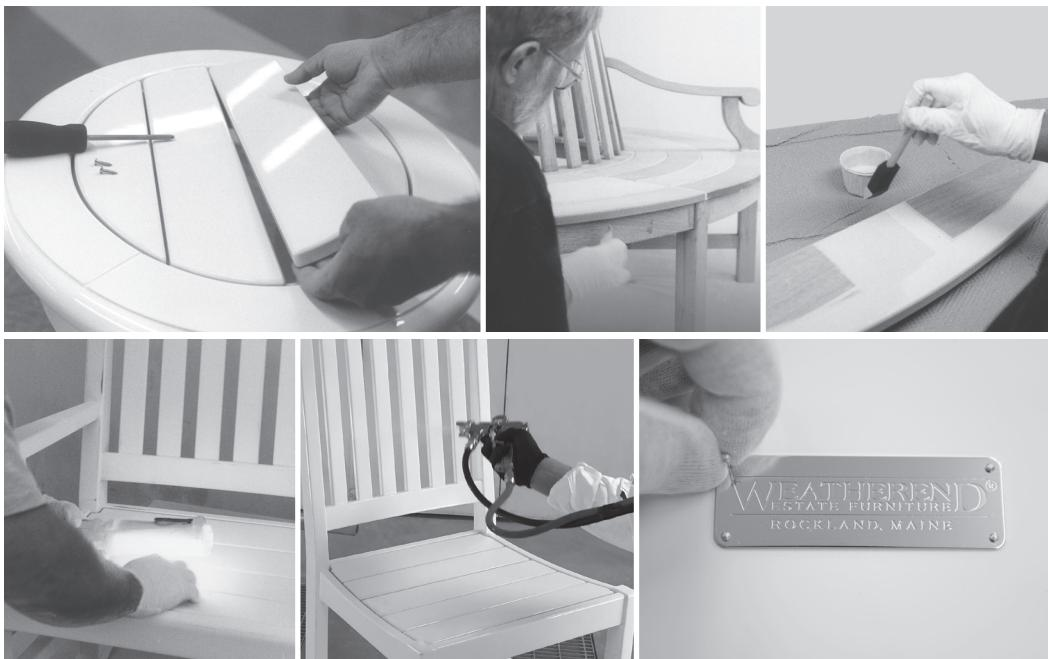
Furniture is disassembled, cleaned, sanded, reassembled with new parts as needed, primed and finished with a total of eight coats of Weatherend Yacht Finish in the color of your choice. Quality Control inspects each piece and a new Product Warranty is provided.
